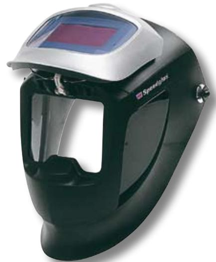
The Speedglas FlexView welding shield has a big, 120 x 90 mm clear visor that is ideal for precision weld preparation under low light conditions. The users simply lift up the spring-mounted welding filter assembly when welding is finished. The spring holds the auto-darkening filter securely on top of the shield, giving the welder a big, clear view behind the FlexView visor.
